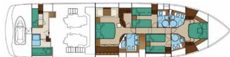
Lower deck Standard version 4 cabins + crew cabin
