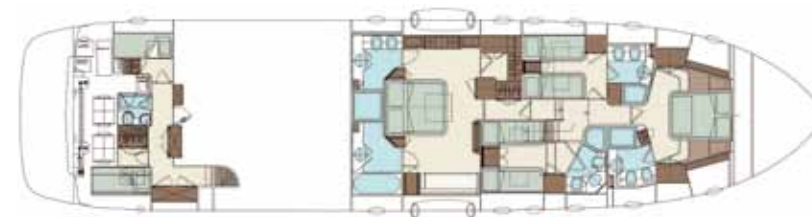
Lower deck Standard version 4 cabins + crew cabin
